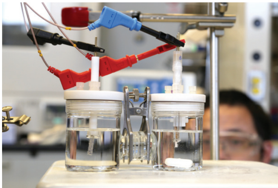
Image from one of the authors showing the electrochemical cell used to test the nickel containing catalysts for the conversion of CO 2 and water into carbon monoxide and oxygen.
